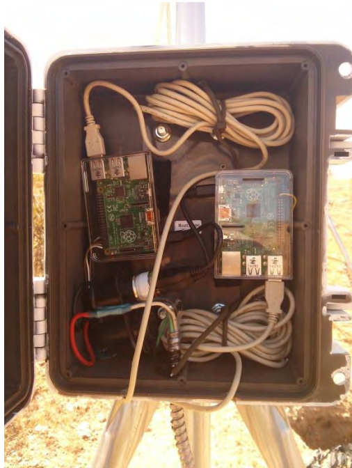
Figure 4 & 5. Left: Microprocessors collecting data. Right: Grand wash Bench Dark Sky Station with the SQM sensor in the tripod towards the rear left
