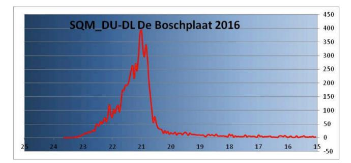
In August 2016 and later in May 2017 the SQM-LU-DL used, is calibrated against a sophisticated device and with all the other SQM used in the Netherlands and for all the Sqm's used a correction is established. The SQM's are gradually getting less sensible and the used SQM LU-DL (number 1985) is corrected for August 2016 with 0,68 magnitude and in May 2017 with 0,7 magnitude.
