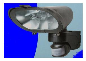
**Good** – Reflector shaped to direct light down. Boxed as dark sky friendly and has PIR sensor separate from the lamp unit pointing. For rural setting look for unit with a 150 watt lamp or less. Also provides reduced illumination dusk to dawn for courtesy and full power on presence detection.
