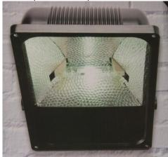
**Good** – (above and below) 70w or 150w metal halide lamp. Must be installed with glass window **horizontal** – **and not as illustrated**. When the lamp is located at the bottom of the reflector the main beam will emerge from the glass window at about 45 degrees. Known technically as a double asymmetric light distribution.
