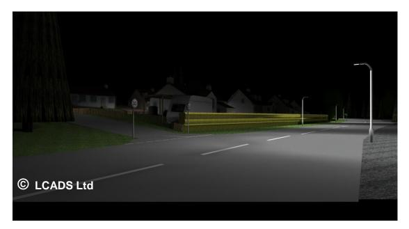
**Figure 1.12:** Luminaires with fully cut-off distribution showing distinct lack of upward spill light detail.
