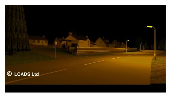
**Figure 1.11:** Traditional Low Pressure Sodium distribution - the luminaire positions were then replaced by luminaires with flat glass and mounted horizontally with an equivalent wattage consumption using LED light sources.
