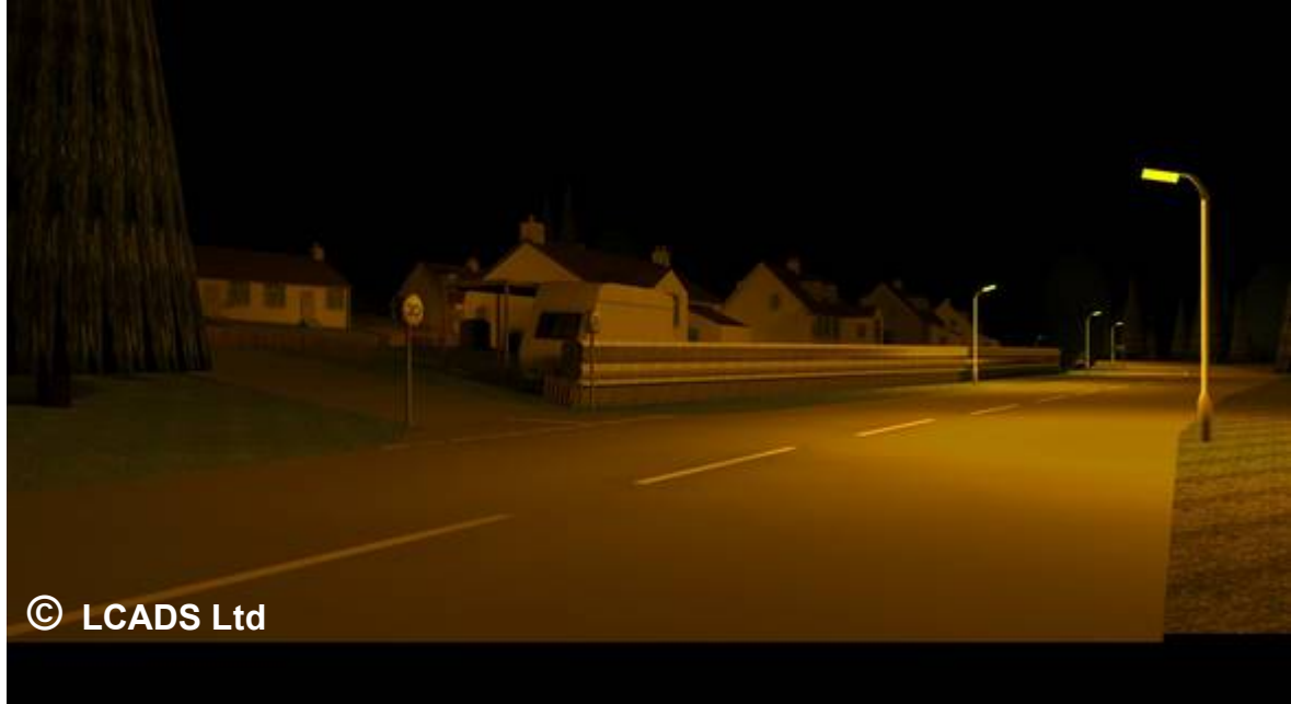
Figure 1.6 Traditional Low Pressure Sodium distribution - shows house details up to chimney pots
