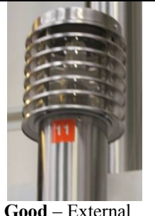
Good – External louvers limit upward light and reduces glare. Lamp must be less than 600 lm
