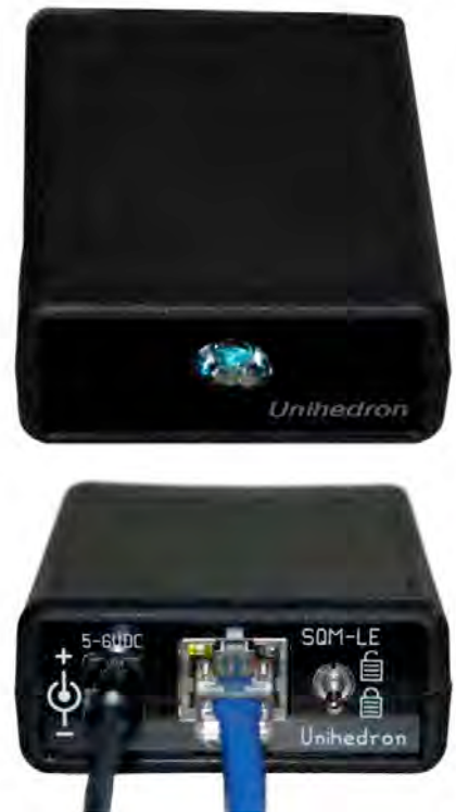
Figure 5. The Sky Quality Meter (SQM-LE) with Ethernet Cable.
