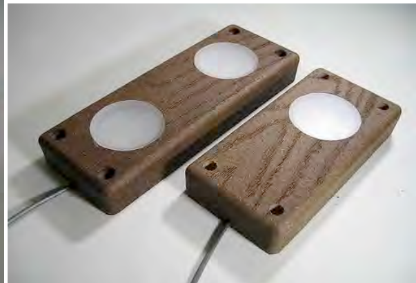
Holly Solar LED Brick, with LED clusters mounted in Trex decking material.
