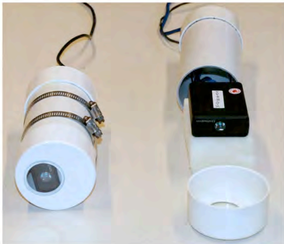
Figure 4. The Sky Quality Meter and the standard weatherproof housing.
