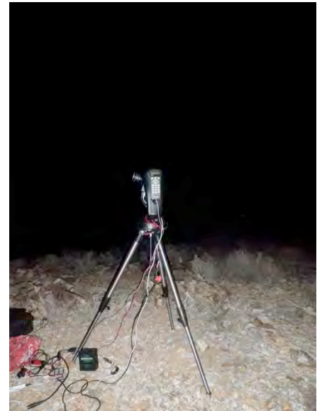
Figure 7. Camera attached to robotic mount and tripod.
