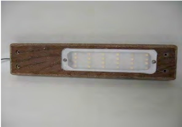
Holly Solar small LED panel mounted in Trex decking
