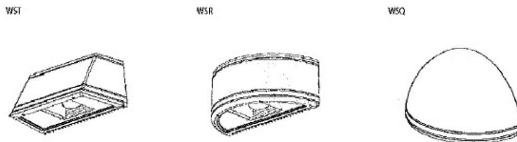
Figure L: Samples of acceptable wall packs.
