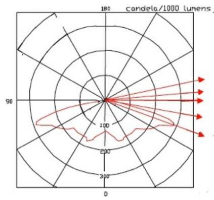
Figure 1.2 - Polar Diagram of typical street lighting luminaire Also shows the angles and maximum intensity values for a "fully shielded (cut-off)" luminaire
